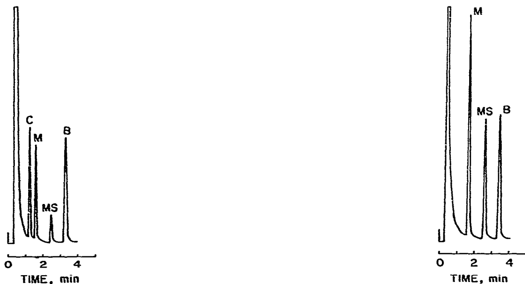
Fig. 3. Gas chromatogram of the extract from a commercial hydrophilic preparation run under conditions described in text. C = camphor; M = menthol; MS = methyl salicylate; and B = benzyl alcohol.
